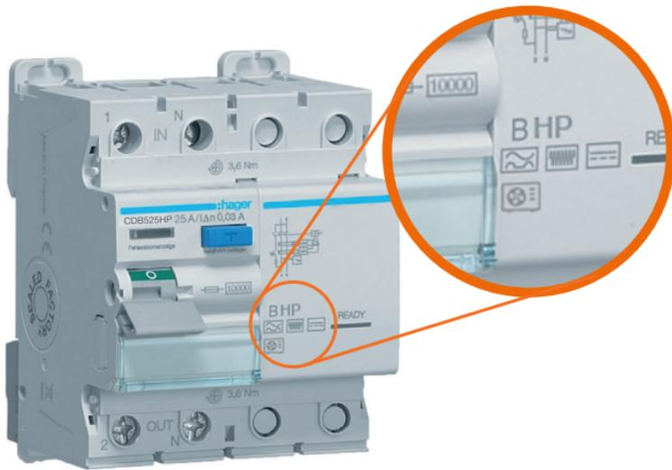
**Hager's Type B HP RCD** takes this a step further by operating at frequencies greater than 20 kHz and maintaining a minimum tripping point of 150 mA for frequencies above 1 kHz. This precision is critical for the reliable and safe operation of heat pumps.
