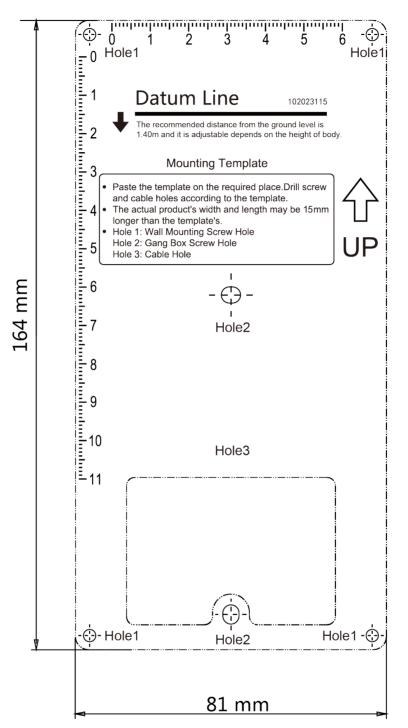
Figure 4-2 Mounting Template
