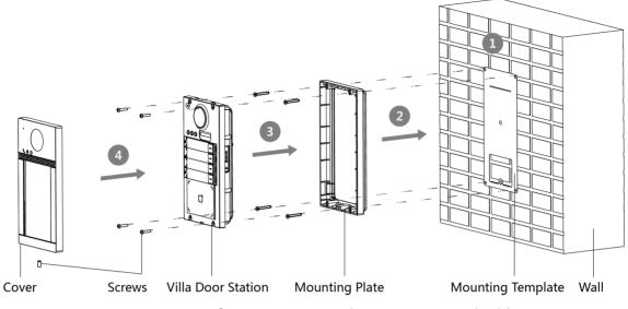
Figure 4-5 Surface Mounting without Protective Shield
