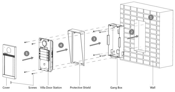
Figure 4-7 Flush Mounting with Protective Shield
