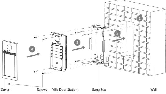
Figure 4-9 Flush Mounting without Protective Shield
