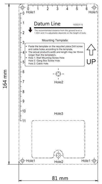
Figure 4-8 Mounting Template
