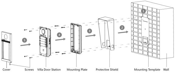
Figure 4-3 Surface Mounting with Protective Shield
