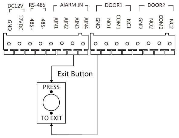
Figure 3-4 Exit Button Wiring
