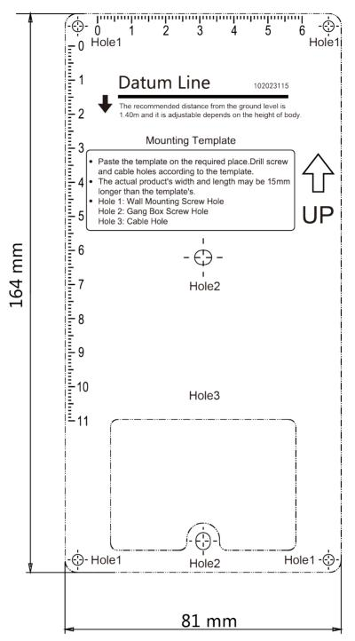
Figure 4-6 Mounting Template
