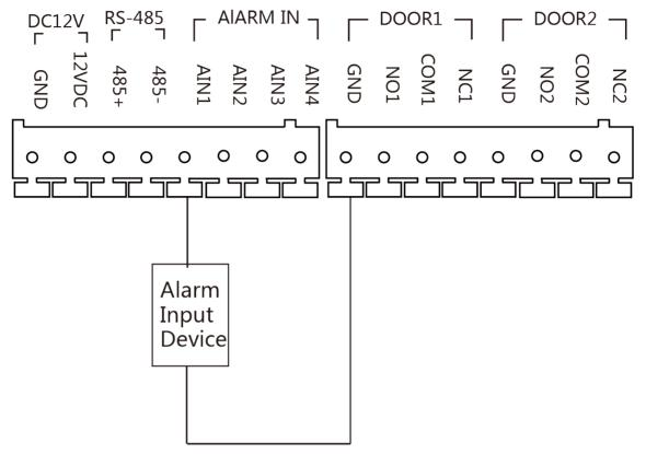
Figure 3-5 Alarm Input Device Wiring
