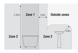
This product is suitable for use in Zone 2 and outside Zones of a bathroom. See diagram.
