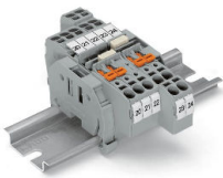
One center and two side marker slots for WMB markers or marking strips Dual jumper slots in the same location as other 2002 Series terminal blocks Commoning options in front of or behind the knife disconnect, depending on the power supply direction
